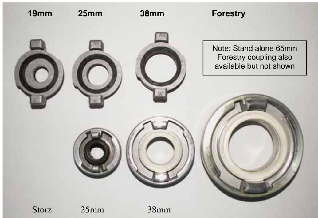
**Storz & Forestry Couplings showing relative size, restrictive nature of Storz coupling compared to size and difference between an internal and external lug connection.**
