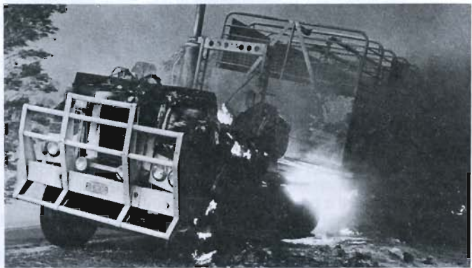
A semi-trailer was gutted by fire on the Glencoe-Kalangadoo road. As fire crossed the road in the path of the truck, the brake line caught fire, stopping the truck and the fibreglass cabin was burnt.
